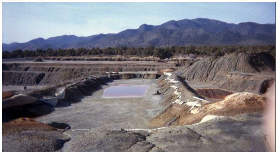
Figure 1 – Tailings with ponded water containing toxic levels of heavy metals.
